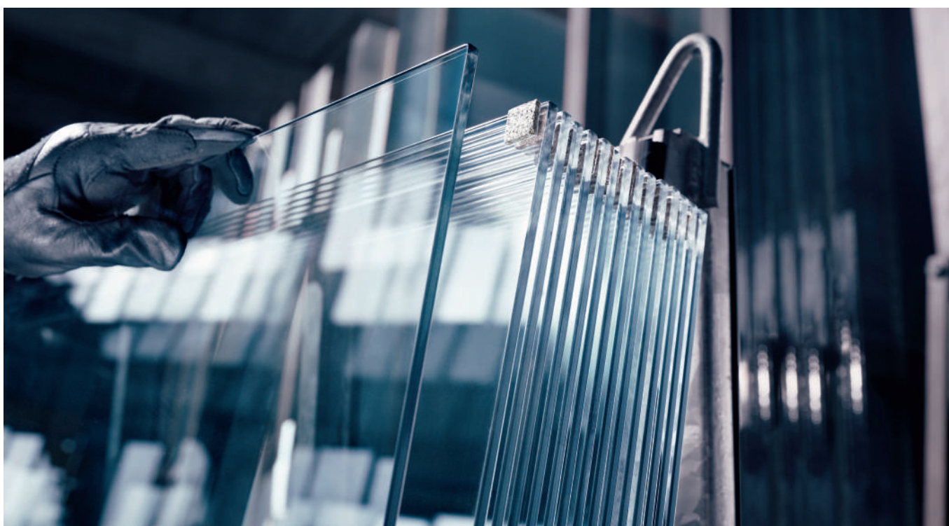
Application Float and laminated glass processed on straight line double edging machines
